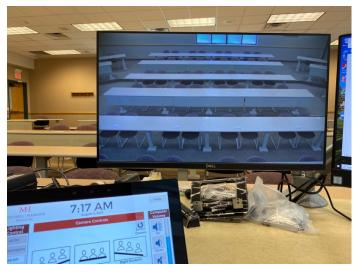
• "Advanced Controls" allows for finite adjusting of the zoom and angles of the classroom camera.
